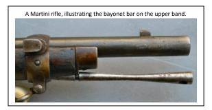
The rifle was made with a bayonet bar on the upper barrel band onto which the slot in the bayonet pommel fit, held in place by a flat spring catch. A muzzle ring set into the bayonet crossguard slid over the end on the barrel, fixing the weapon securely to the rifle.
