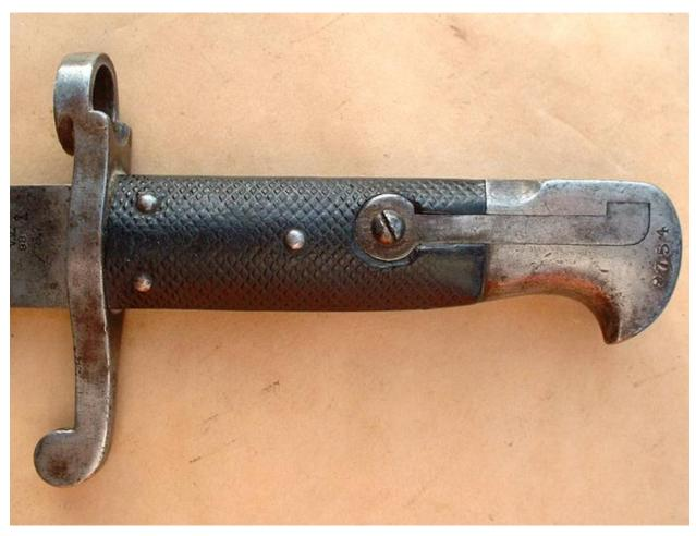
P1887 Mk.I bayonet with replaced, new 'stepped' muzzle ring
